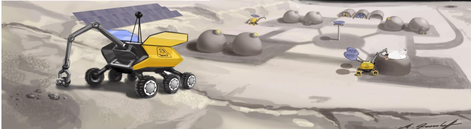
A lunar rover equipped with a 3D printer, which will be used to collect building materials on the moon and for on-site printing tests.
